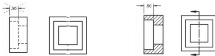
Figure 10.1: Sectioning facilitating dimensioning
