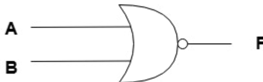
Figure 9.5: Two-input NOR Gate
