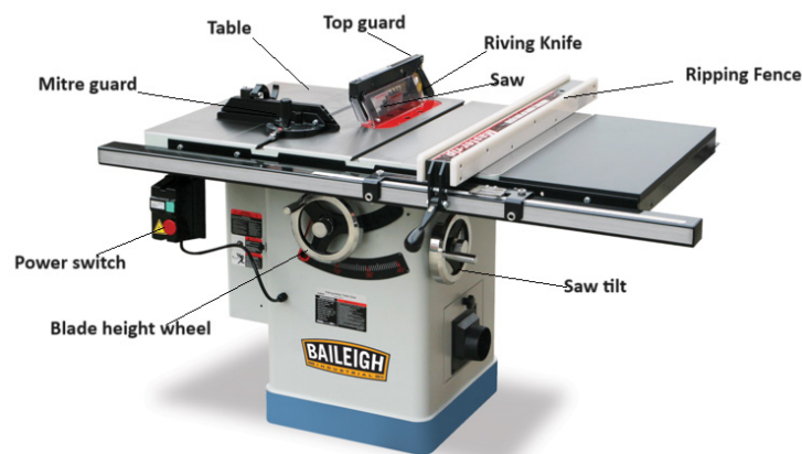
Figure 2.2: Circular saw bench main parts
