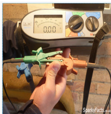
Figure 3.11: Setting the meter
