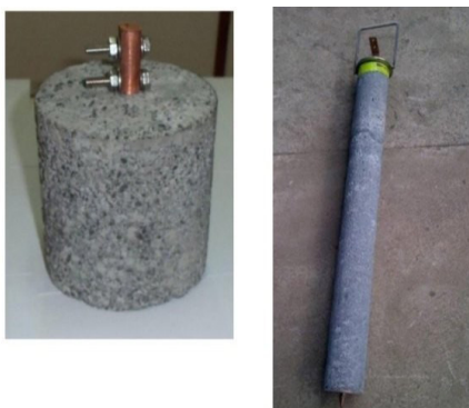
Figure 3.6: Marconite earthing compounds
