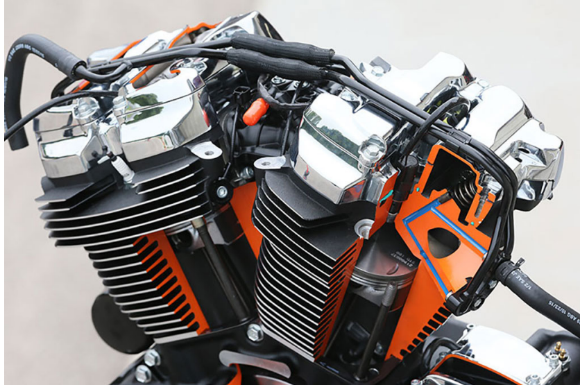
Figure 1.1.2: Cooling fins on a typical air-cooling system
