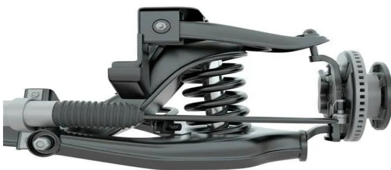
Figure 5.17.6: Independent suspension arrangement
