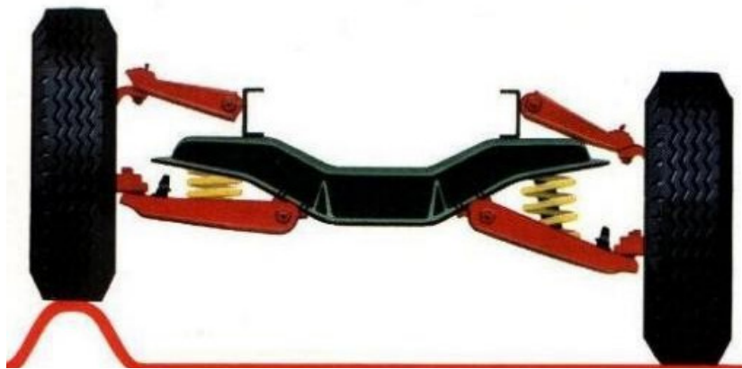
Figure 6.21.2: Independent suspension system.
