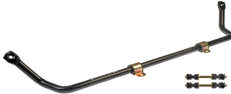
Figure. 5.17.4: A stabiliser bar.
