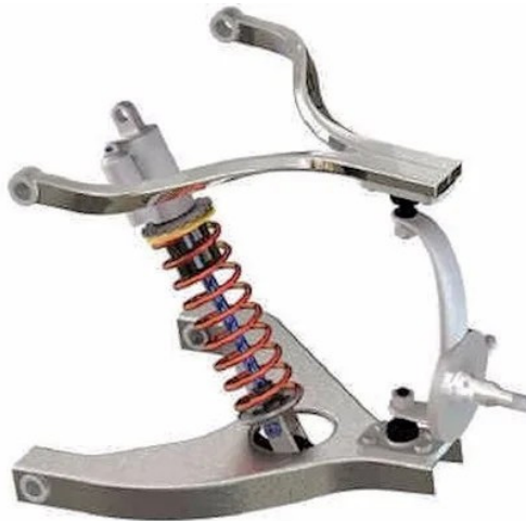
Figure 6.21.4: Double-wishbone arm linkage
