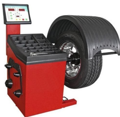
Figure 6.23.14: A wheel tyre balancing machine
