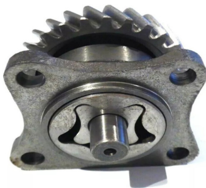
Figure. 2.7.8: Gear-type oil pump
