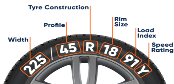
Figure 6.23.11: Tyre sidewall markings
