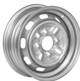
Figure 6.23.1: A pressed steel wheel
