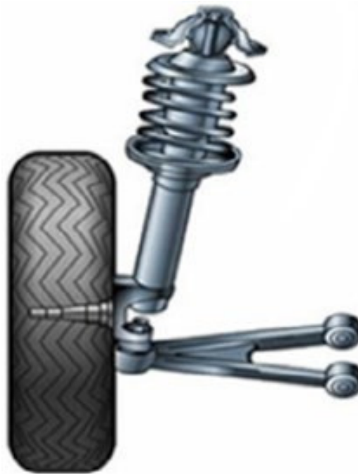
Figure. 6.21.6: Macpherson strut linkage
