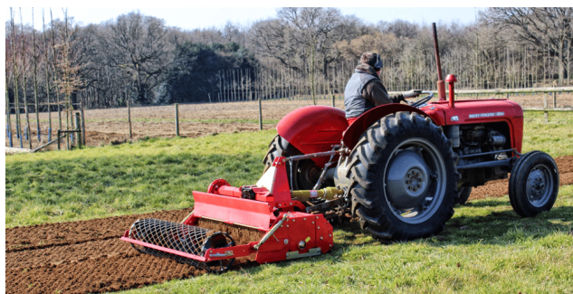
Figure 4.2: Tractor-mounted rotatory tiller
