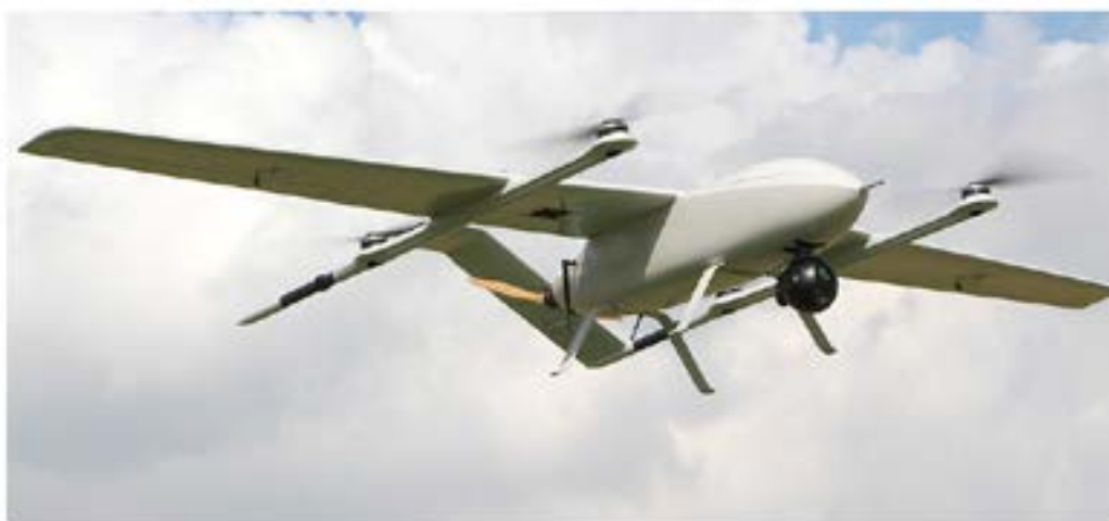
Figure 6.3: FW320 VTOL UAV (Long Endurance VTOL Drone | 23KG MTOW | 2.5Hours Endurance)
