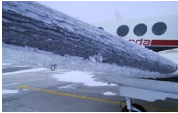
Figure 1.15: Ice formation on aircraft wing (NTSB Calls For FAA, GAMA To Work On New Aircraft Icing Alert System – Disciples of Flight)
