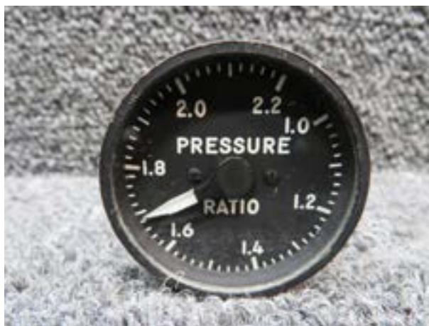
Figure 4.19: Engine pressure ratio indicator (Source: Bendix )
