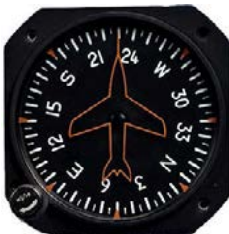
Figure 4.7: Heading indicator (Source: Pilot Workshop )
