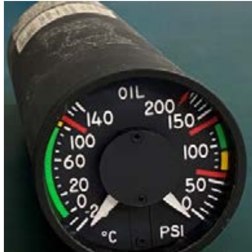
Figure 4.14: Shared oil temperature and pressure display (Source: Aviation Instrument Service )
