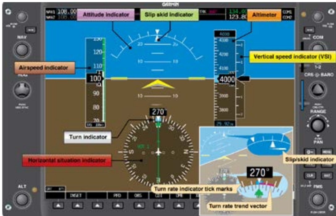
Figure 4.9: Primary flight display (Source: Pilot's Handbook of Aeronautical Knowledge )
