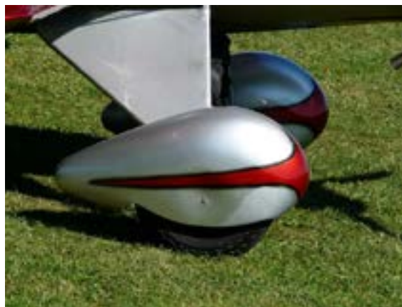
Figure 2.44: Faring on a non-retractable landing gear
