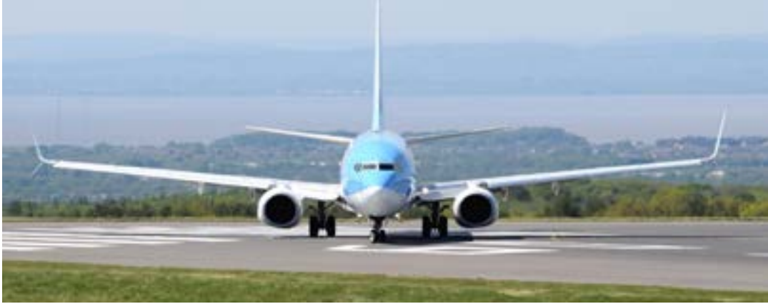
Figure 2.28: Dihedral wing and tail plane of the Boeing 737-800 ( Wing Nomenclature )
