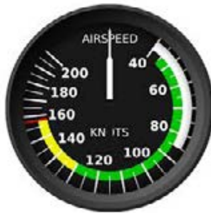
Figure 4.2: Airspeed indicator (Source: Flight Nerd Air Force )
