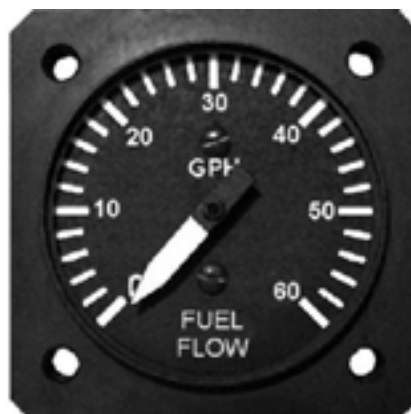
Figure 4.18: Aircraft fuel flow meter (Source: Aircraft Spruce and Specialty Company )
