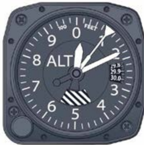
Figure 4.4: Altimeter (Source: Flying Magazine )
