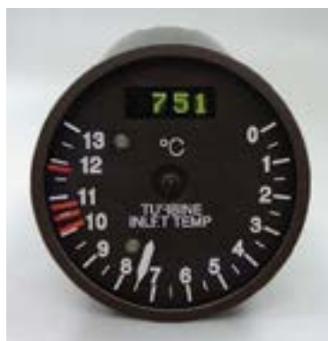
Figure 4.20: Turbine inlet temperature gauge (Source: Innovative Solutions and Support )
