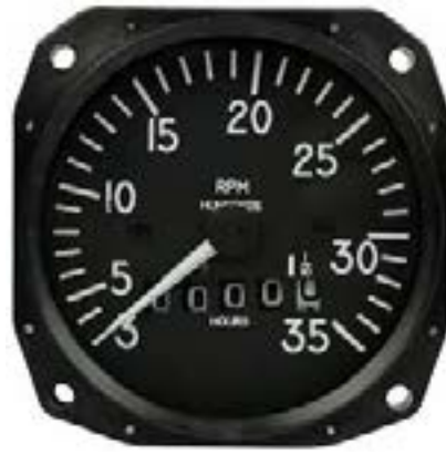
Figure 4.10: Aircraft tachometer (Source: Aircraft Spruce and Specialty Company )
