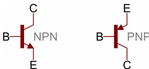
Figure 4.16.3: Direction of current flow
