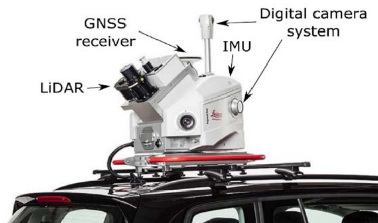
Figure 7.12: Mobile Mapping Systems with sensors and devices mounted on a vehicle (MDPI)
