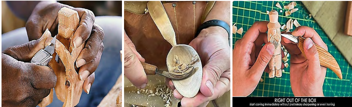
Figure 5.110: Whittling technique of carving
