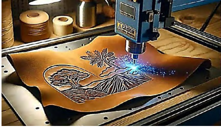
Figure 5.118: Laser Engraver on Leather
