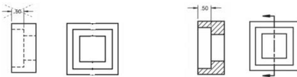
Figure 3.73: Sectioning facilitating dimensioning
