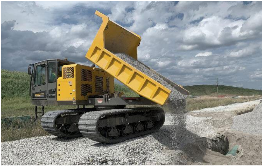
Figure 7.22: Crawler (Tracked vehicle)
