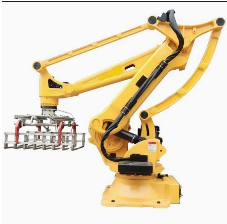
Figure 7.1: Crane with a mechanical arm showing a closed loop mechanism
