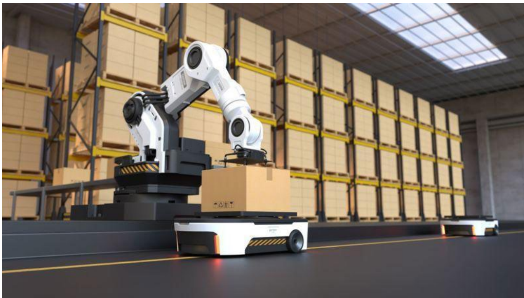
Figure 7.6: Warehouse robot with a closed chain arm designed for lifting
