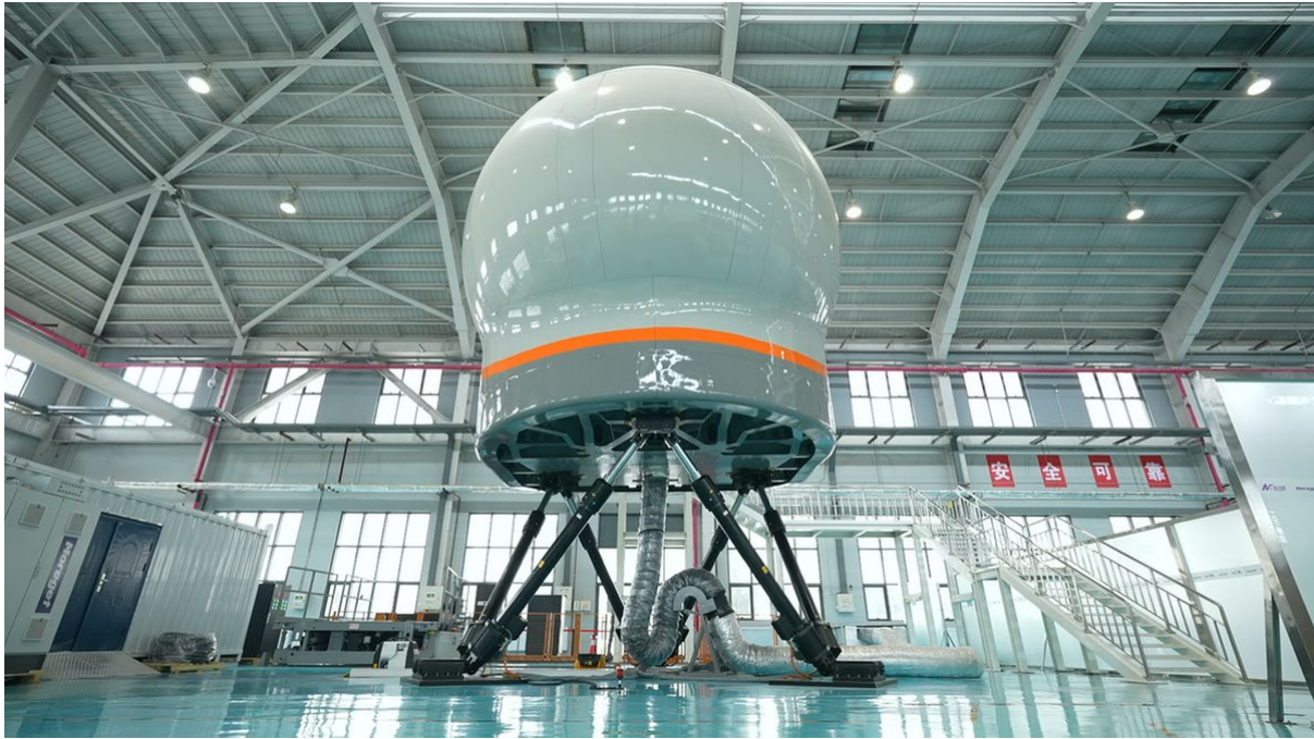
Figure 7.7: Flight simulator using a closed chain mechanism
