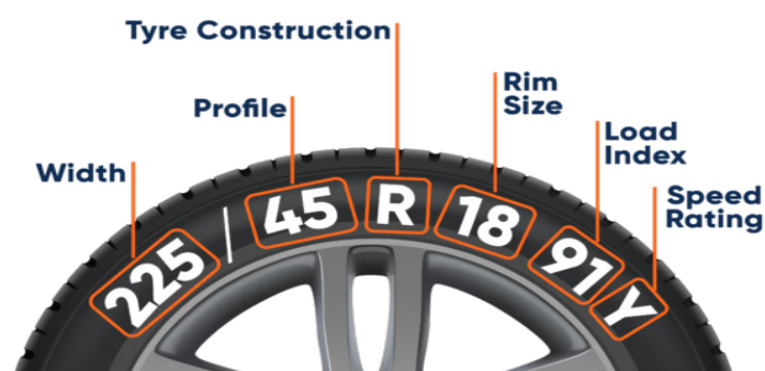
Figure 23.11: Tyre sidewall markings
