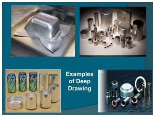
Figure 20.3: Some products of deep drawing
