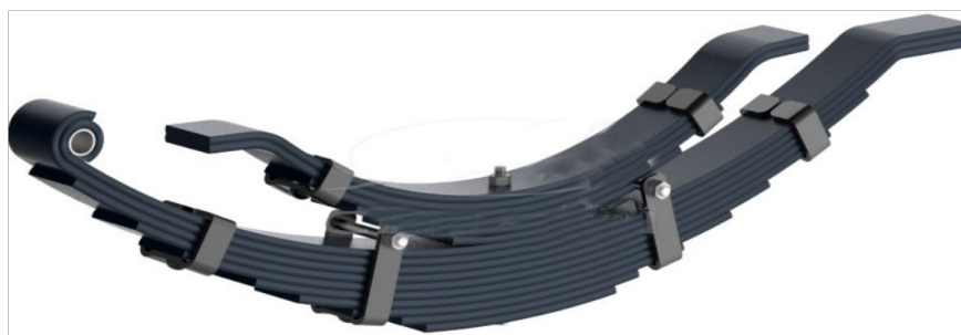
Figure 19.3: A Leaf spring with a helper spring.
