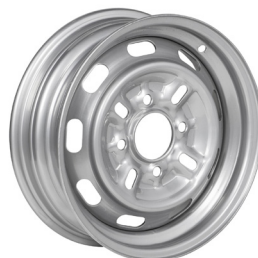
Figure 23.1: A pressed steel wheel
