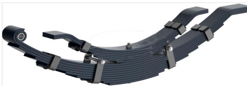
Figure 19.3: A Leaf spring with a helper spring.
