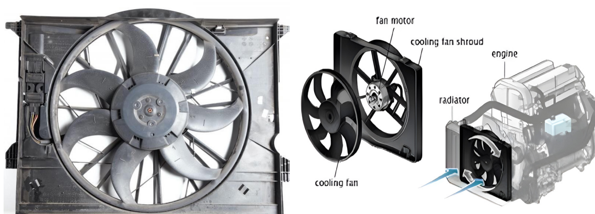
Figure 3.5: Radiator fan with labelled parts and fan fixed to an engine
