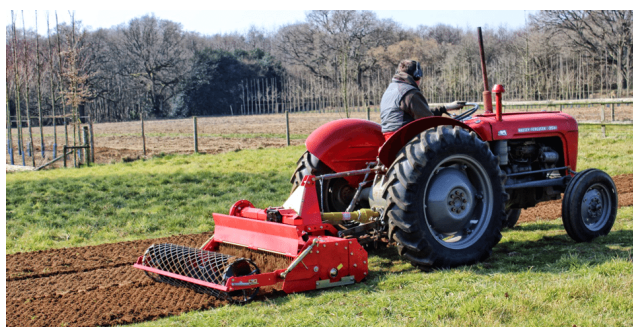
Figure 4.2: Tractor-mounted rotatory tiller
