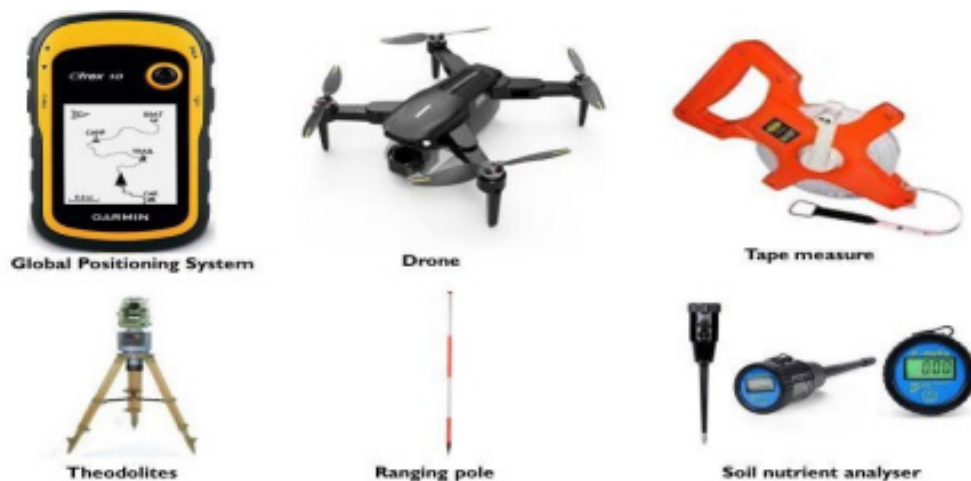
Figure 3.3: Some Survey and Mapping Instruments
