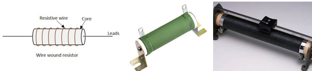
Figure 4.13.4: Resistors – wire wound, fixed wire wound and variable wire wound
