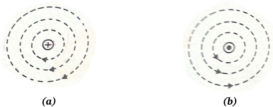
Figures 6.22.3: (a) Field of current flowing away from observer. (b) Field of current flowing towards observer.
