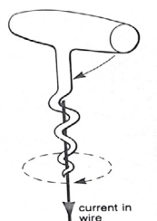
Figure 6.22.2: a corkscrew showing direction of current and magnetic field
