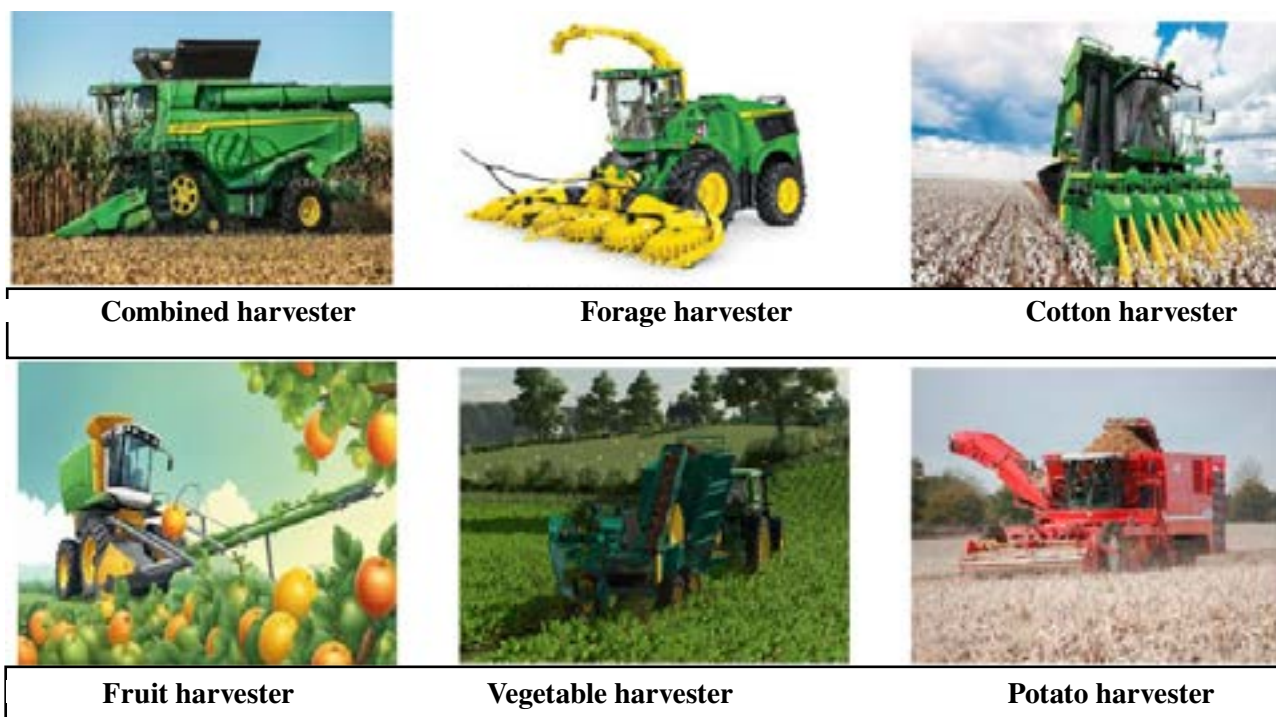
Figure 9.2: Some Mechanised Harvest Tools
