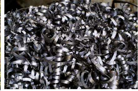
Fig. 16.4: Metal shaving from lathing
