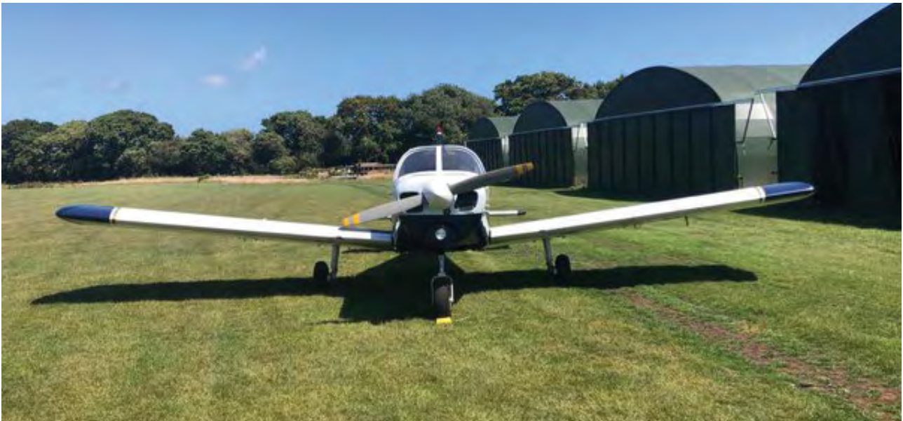
Figure 28: Aeroplane with dihedral wing
