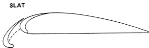
Figure 21: A leading-edge slat.
