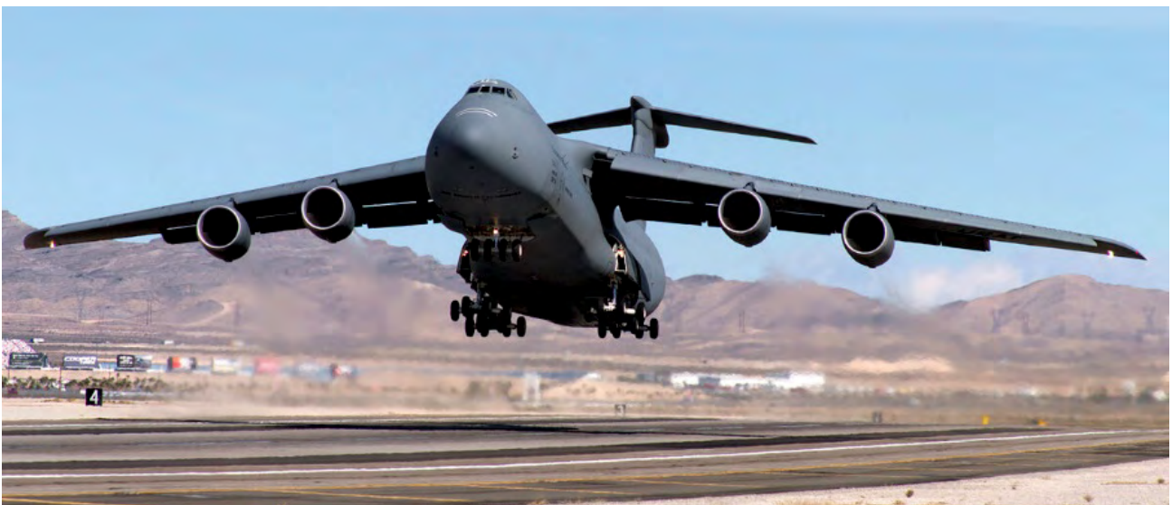
Figure 30: Military cargo aeroplane with anhedral angle
