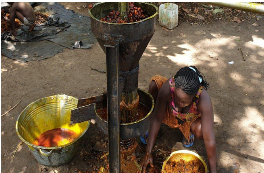
Figure 11.1: Palm oil processing using simple machines
