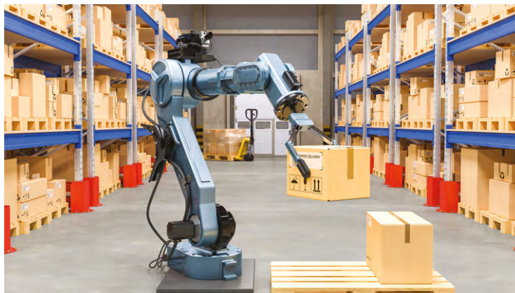
Figure 18.6: Warehouse robot with a closed chain arm designed for lifting.
