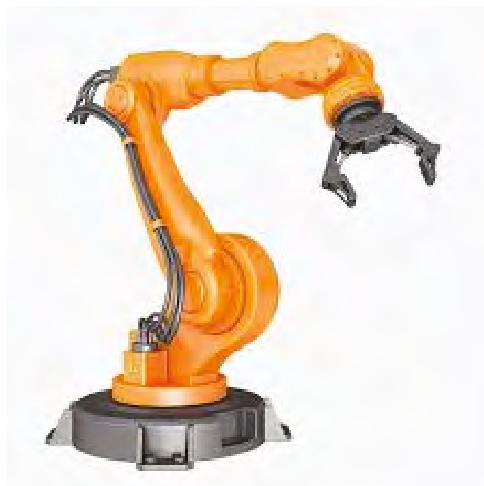
Figure 18.1: Robotic arm showing closed loop mechanism
