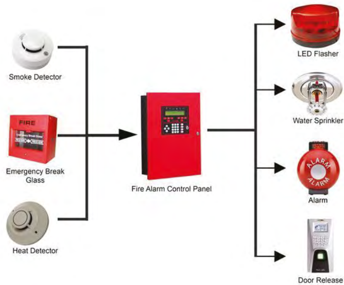
Figure 3.1: Component Diagram of a Fire Alarm system
