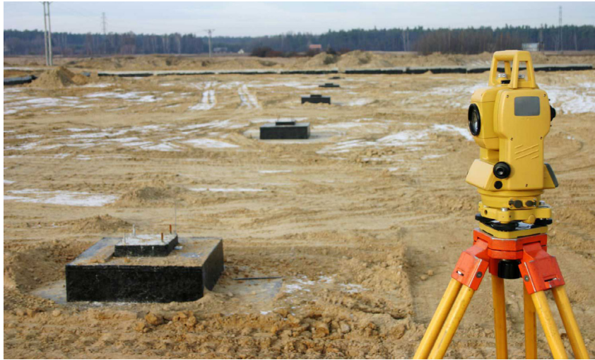
Figure 1.52: Theodolite mounted on a tripod and fitted with an EDM
