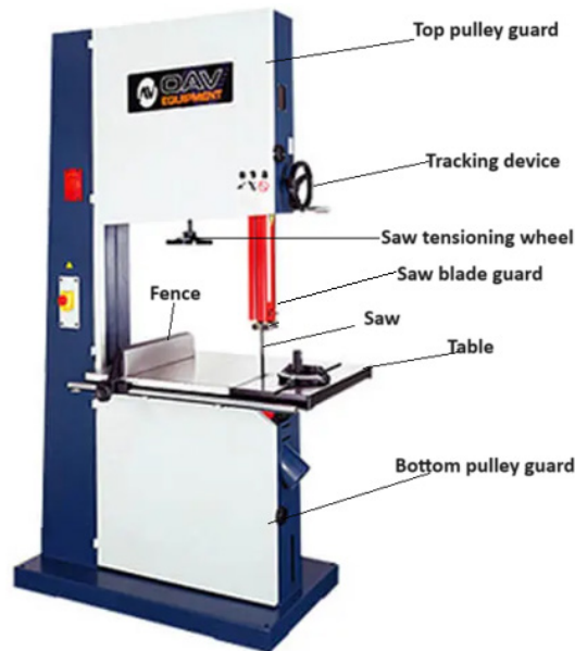
Figure 2.8: Narrow bandsaw main parts
