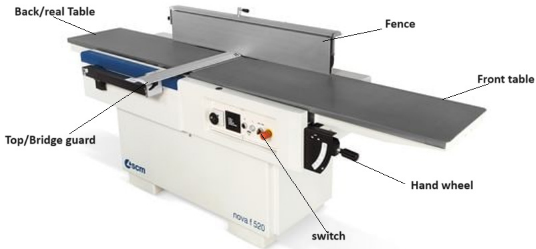
Figure 2.9: Surface planer main parts
