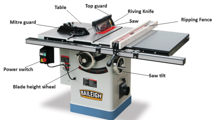
Figure 2.2: Circular saw bench main parts
