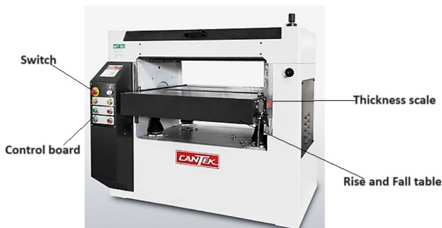
Figure 2.10: Thicknesser machine main parts
