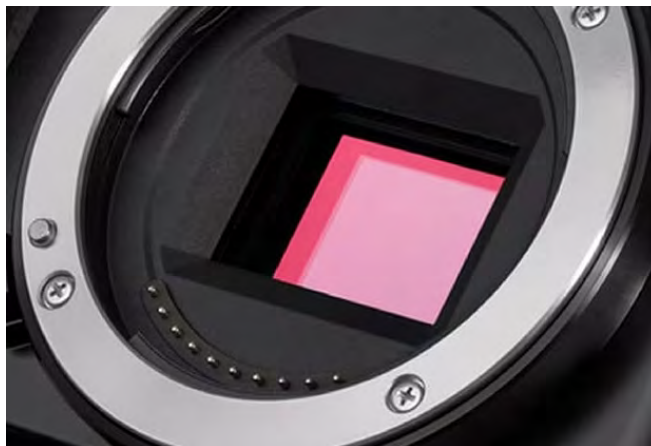
Figure 39: Instead of a photographic film, a digital camera uses a CCD to capture images
