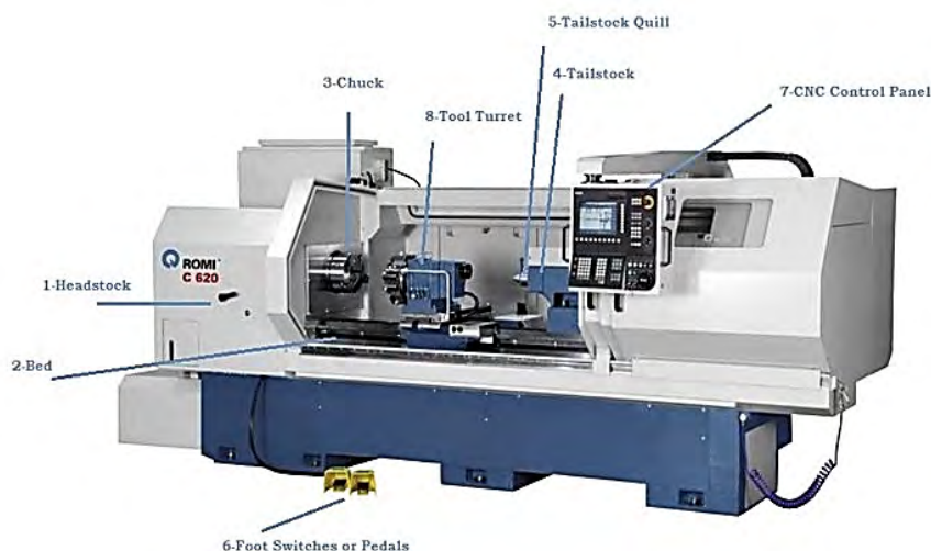
Figure 3.2: Main Parts of the CNC Lathe Machine
