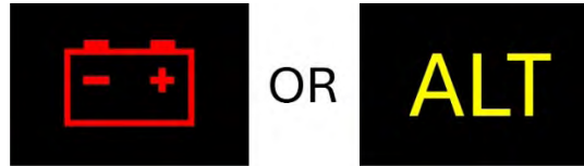
Figure 10.7: Battery charging symbol
