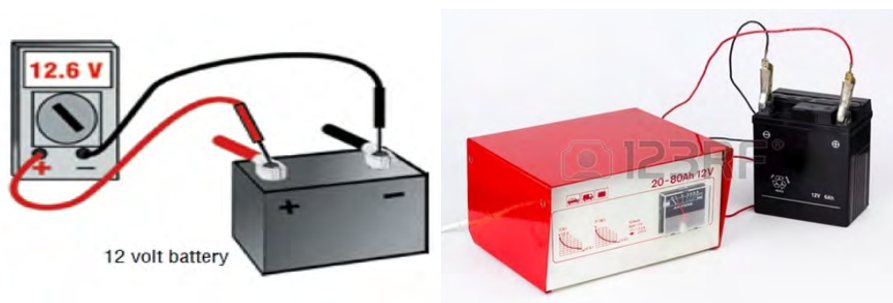
Figure 3.8: Charging of battery with terminal connection
