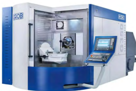
Figure 1.9: Horizontal machining centre
