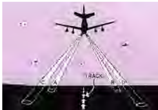
Figure 3.6: Doppler navigation system showing beams
