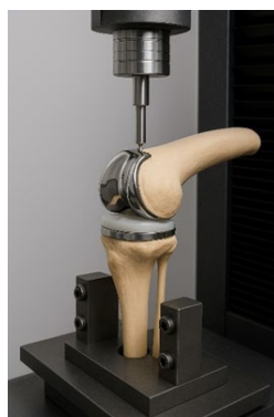
Figure 5.19: Machine testing a knee implant
