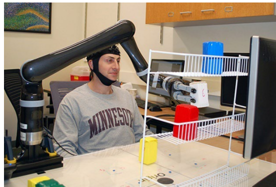
Figure 5.7: Controlling a robotic arm with thought.
