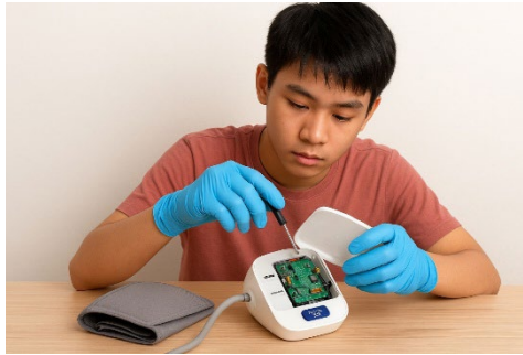
Figure 5.15: Disassembling a digital blood pressure monitor
