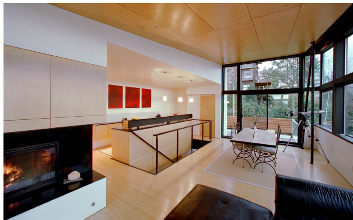
Figure 5.20.4: Plywood boards used for the ceiling.
