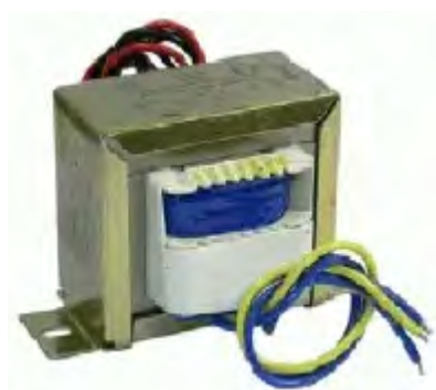
Figure 4.6: A picture of a step-down transformer for electronic circuits.
