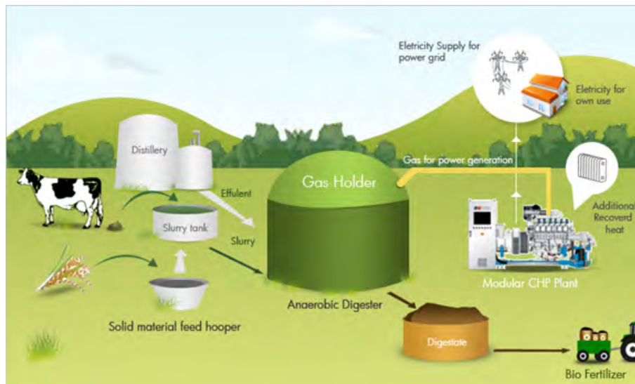
Figure 5.15: Picture of Biogas Energy Output System
