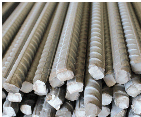
Figure 5.3: Metal rods (Rebar)
