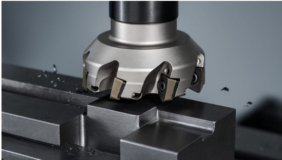
Figure 6.21: A milling cutter held in the tool post performing face milling on a workpiece https://www.3erp.com/blog/face-milling/
