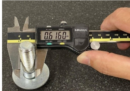
Figure 7.19: A calliper for measuring a component, with tolerance limits marked.
