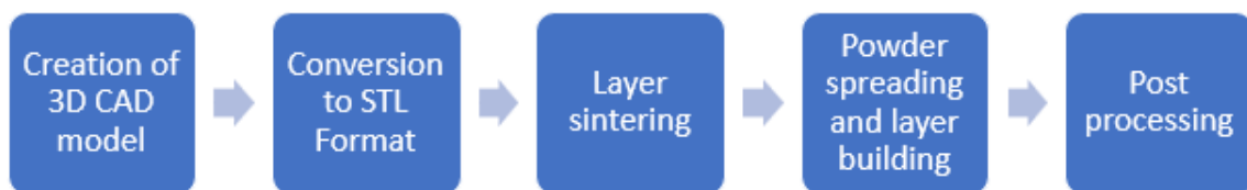
Figure 4.9: Step-by-step process of powder-based prototyping
