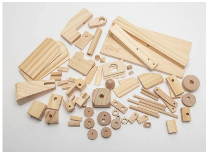
Figure 5.2: Simple wood patterns
