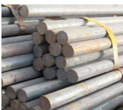
Figure 5.7: Mild steel rods
