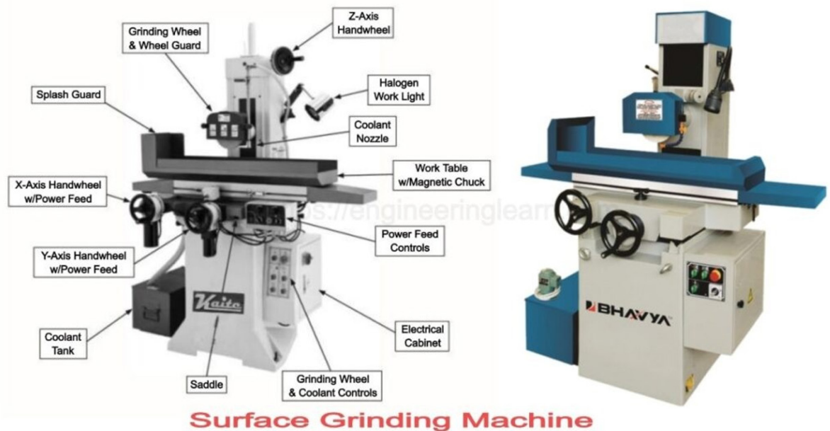
Figure 6.22: Showing a surface grinding machine with labelled parts
