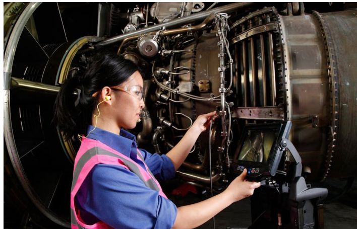
Figure 4.8: Borescope being used for an internal inspection
