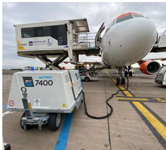
Figure 4.11: Aircraft connected to Ground Power Unit (GPU)
