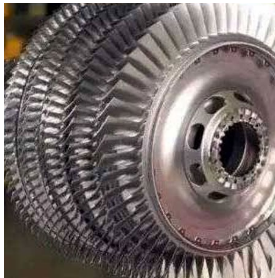
Figure 1.2: Engine components made with titanium alloys
