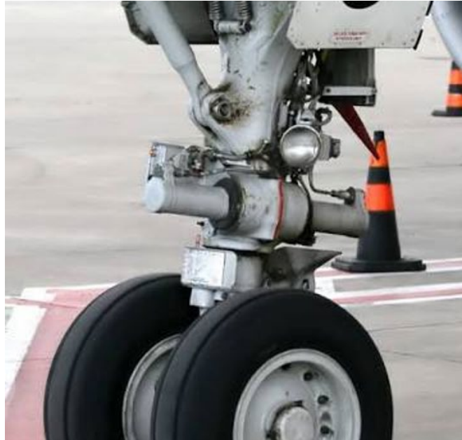
Figure 1.3: Landing gear made of steel alloys
