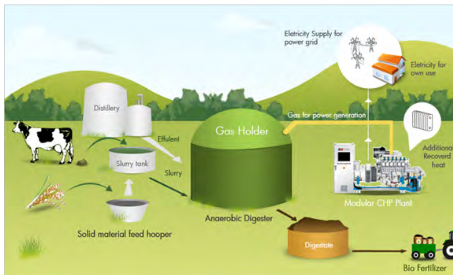
Figure 23: Biogas Energy Output System
